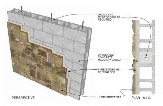
Applying over clean, untreated new masonry. Masonry that is not new/clean/untreated should be cleaned and/or sandblasted to the original surface or covered with metal lath that is securely fastened.
